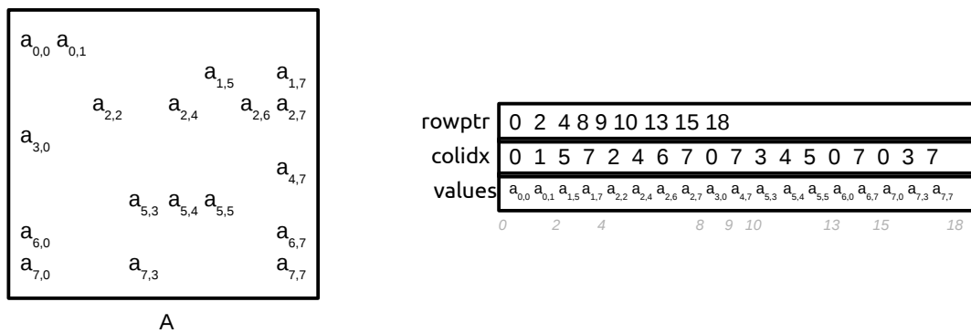
Figure 2.2: CRS matrix storage: the rowptr array gives the offset position of the NNZ in the colidx and values arrays, these two arrays contains the values and their corresponding column indexes in row major.
