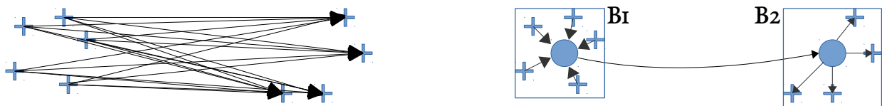
Figure 2.14: The interactions between particles are replaced by interactions using clusters, thus leading to N_1 + N_2 interactions instead of N_1 \times N_2 .
